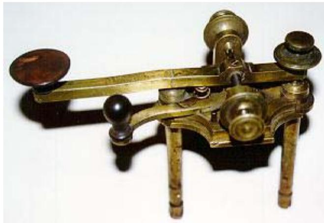
This early straight lever key was made by the Caton Instrument Co., Ottawa, Ill. The long legs pass through holes in the operating table and wires are attached to binding posts at the end of each leg. Circa 1860's
