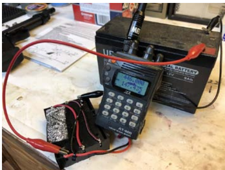
Crossband FM Repeater testing
