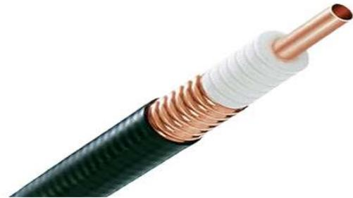
Note the hollow center conductor to save weight and cost. Taking advantage of the RF skin affect .
