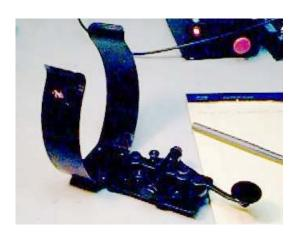
The J45 key is fairly common-- it's actually a J37 key mounted on a spring steel leg clamp for use on aircraft, in tanks, etc. This one is marked J45 on the leg band, stamped J37 on the base of the key, and carries the inscription "SC480A" in red on the back of the leg clamp. The key is black, with a brass finish. Shown here, the key is hinged for use on a desk-- it flips over for use when clamped on the operator's leg.
