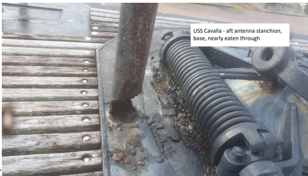
Corroded stanchion base, holding the main wire antenna on the Cavalla. It's to be replaced. Photo by Rick Wannall
