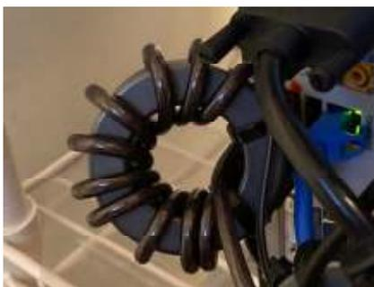
In toroid lexicon, the first number, 240, indicates the diameter, 2.4 inches, while 31 identifies the chemical mix of the ceramic core. The two most popular mixes for ham radio are apparently 31 and 43, where 31 works best for the lower frequencies, 40 meters and below, and 43 is best for those above that.
