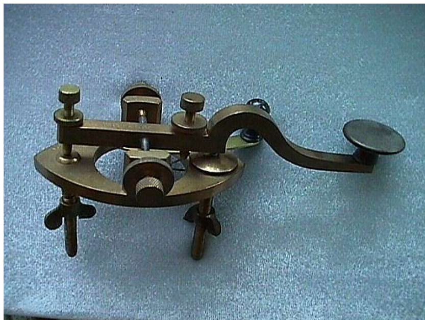
Phelps Camelback Key: Circa 1860 The “camel’s hump” was supposed to give it a better-balanced feel.
