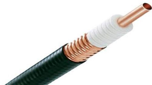
Note the hollow center conductor to save weight and cost. Taking advantage of the RF skin affect .
