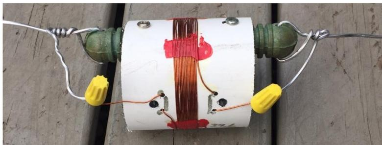
In using the #20 coil, I mounted the pvc coil stock on a long dog bone insulator and configured it as in the picture with temporary wire-nut connections. The antenna can then be put together using the wire lengths in part 1, ensuring good mechanical and electrical connections. I am not a fan of supporting a dipole only at the ends, as the center feed coax
