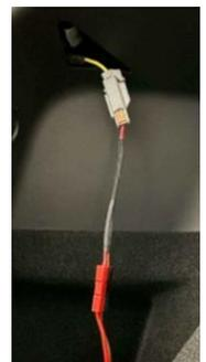
Best yet, they had one in stock for about \$4; a great price for me. I picked it up and took it home, where I cut off the socket and attached a pair of Power Pole connectors to the two wires. I now have the solution for power for the mobile rig in a Tesla. I connected the socket to the wiring harness plug, routed this short cable through the existing emergency trunk release hole then connected it to my mobile rig’s in-line fused power cable.
